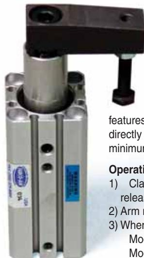
The clamp arm rotates 90° as it extends away from the workpiece providing clearance and access for unload/load operations. Double acting operation and standard magnetic piston offer positive cycles, durability and workpiece detection features. Extruded aluminum body mounts directly and rigidly to equipment surfaces in a minimum of space.
